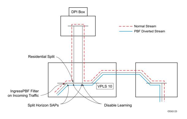
Figure 28: Policy-Based Forwarding for Deep Packet Inspection
